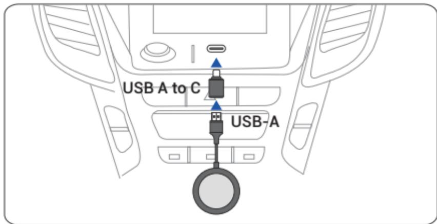
**NOTE!** The adapter should be plugged into the USB port that is for wired Apple CarPlay connecting if there are multi USB ports in your car.
