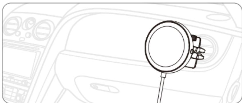
5. Attach the product to the vehicle's air vent using the stand
