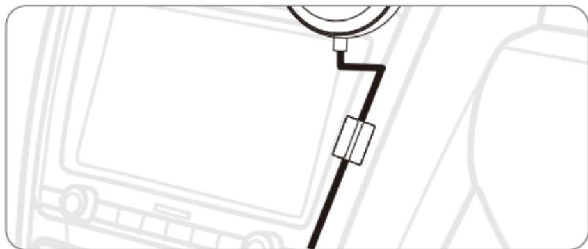
6. The data cables can be organized more aesthetically using cable clamp.
