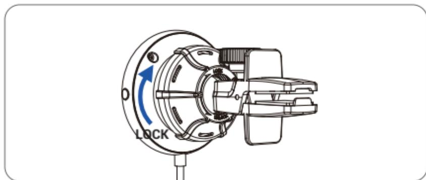
4. Tighten the back cover to complete the assemble
