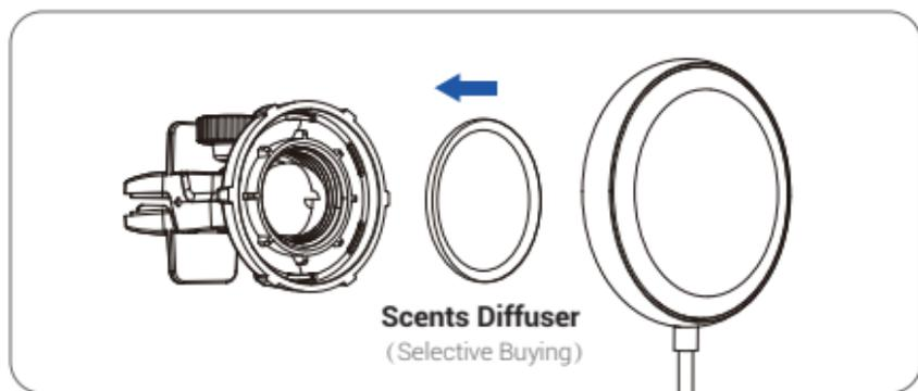
3. Place the diffuser into the back cover
