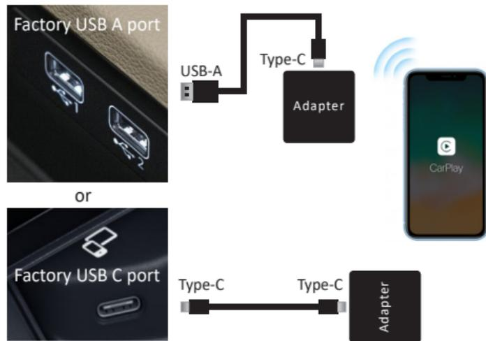
**NOTE!** The adapter should be plugged into the USB port that is for wired Apple CarPlay connecting if there are multi USB ports in your car.
