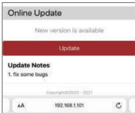
**NOTE!** The red and blue indicator lights will flash alternately while updating. Wait for more than 30s after light is always on, then disconnect and reconnect the adapter from the USB port to finish the whole update.
