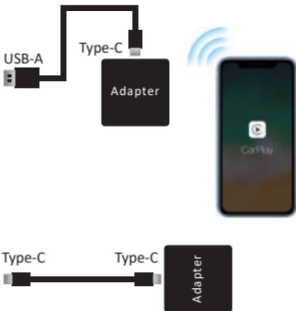
**NOTE!** The adapter should be plugged into the USB port that is for wired Apple CarPlay connecting if there are multi USB ports in your car.
